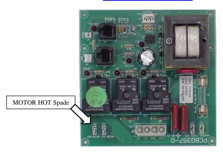
The other end of the inrush limiter will attach to the PWM (motor control) board at the spade marked "L2". See the diagram below.
