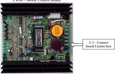
After attaching the inrush limiter to the correct spades, bend the wires of the inrush limiter so that they are out of the way of any fans or moving parts. The black, nickel-sized resistor on the inrush limiter will get very hot while in use, so make sure it does not rest on or touch any other parts under the hood. As always, if you have any questions or problems, please contact the service department at Noramco Fitness.
